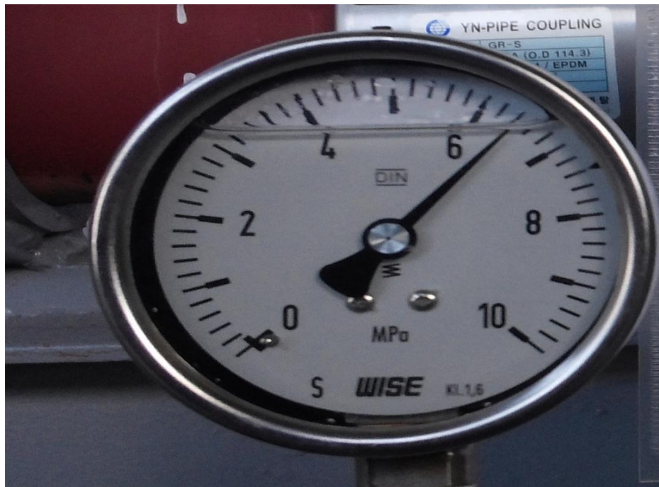
Photo 3-2. The Pressure of Burst Pressure Test
